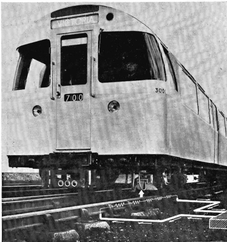
One of the carriages of London's new Victoria Line underground railway. The diagram, lower right, shows how trackside signalling equipment passes signals to the train's automatic control. These messages are picked up by coil (arrowed) just above the track.
