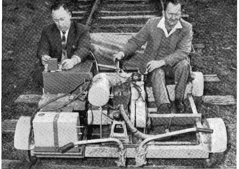
The Rail Flaw Detector Car uses magnetic as well as ultra-sonic methods of detecting flaws. Two other cars of an improved type are in course of construction.
