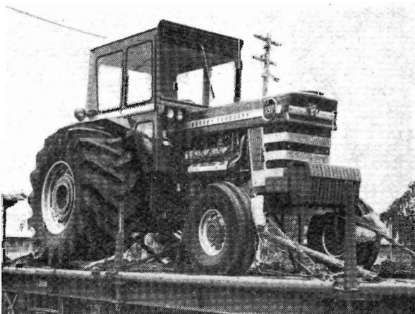
The hydraulic crane bound for Kewdale, W.A. and the tractor consigned to Parkes, N.S.W. had one thing in common. They were both out of gauge until the wheels were removed from the crane and the exhaust pipe from the tractor.
