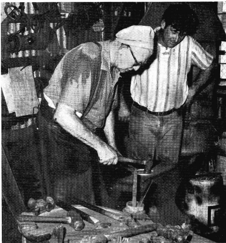
Watched by his son, Mr. Edmunds finishes a horse-shoe on the anvil.
